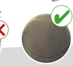
Sample taken from an oil-less compressor with dryer – dry air eliminates the risk of bacterial growth.
